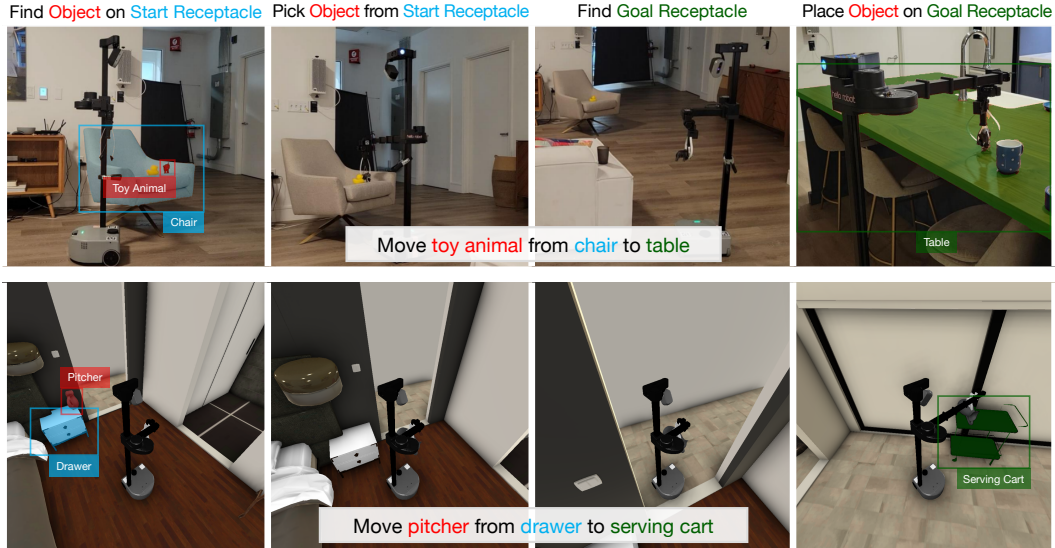
Figure 1: Open-Vocabulary Mobile Manipulation requires agents to search for a previously unseen object at a particular location, and move it to the correct receptacle.
