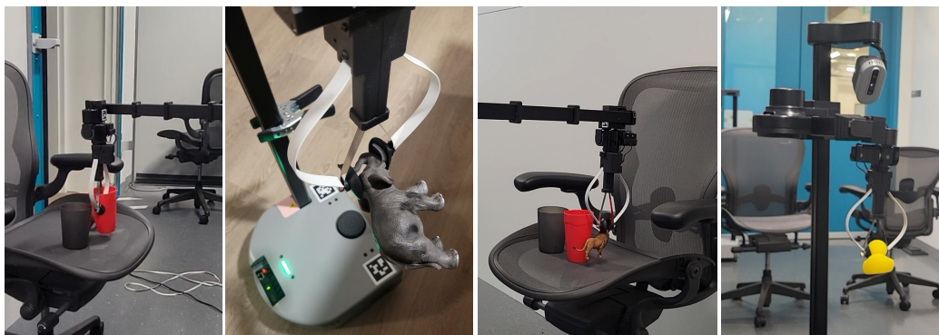
Figure 13: Grasping tests in various lab environments. To provide a strong baseline, we tuned the grasp policy to be highly reliable given the Stretch’s viewpoint, on a variety of objects.
