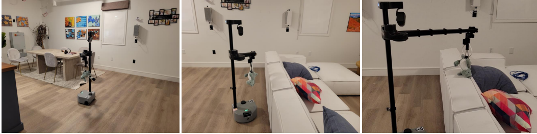
Figure 14: An example of the robot navigating to a goal_receptacle (sofa) and using the heuristic place policy to put down the object (stuffed animal). Heuristic policies provide an interpretable and easily extended baseline.
